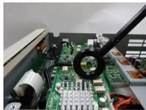
The measurement of conventional magnetic field probe
