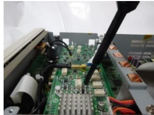
The measurement of conventional electric field probe
