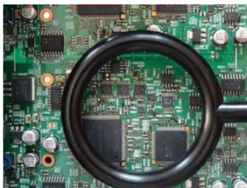
General loop magnetic probe , diameter: 6.8cm
