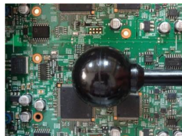
General sphere electric probe, diameter: 3cm
